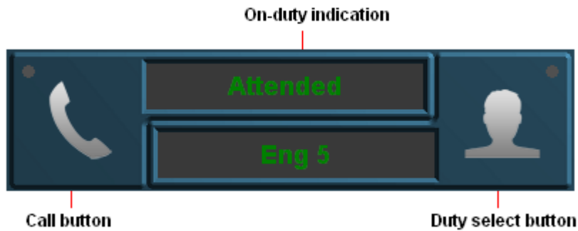
Figure 2-25: Call button / on-duty indication / duty select button
