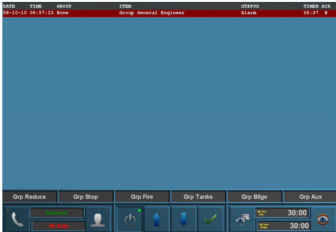
Figure 2-20: Alarm panel screen (incl. on-duty selection)
