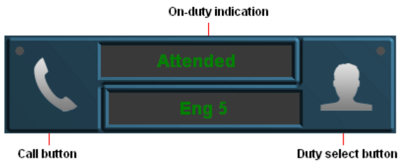
Figure 2-22: Call button / on-duty indication / duty select button
