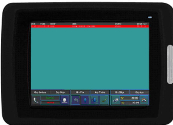
Figure 2-24: Duty alarm panel (DAP)
