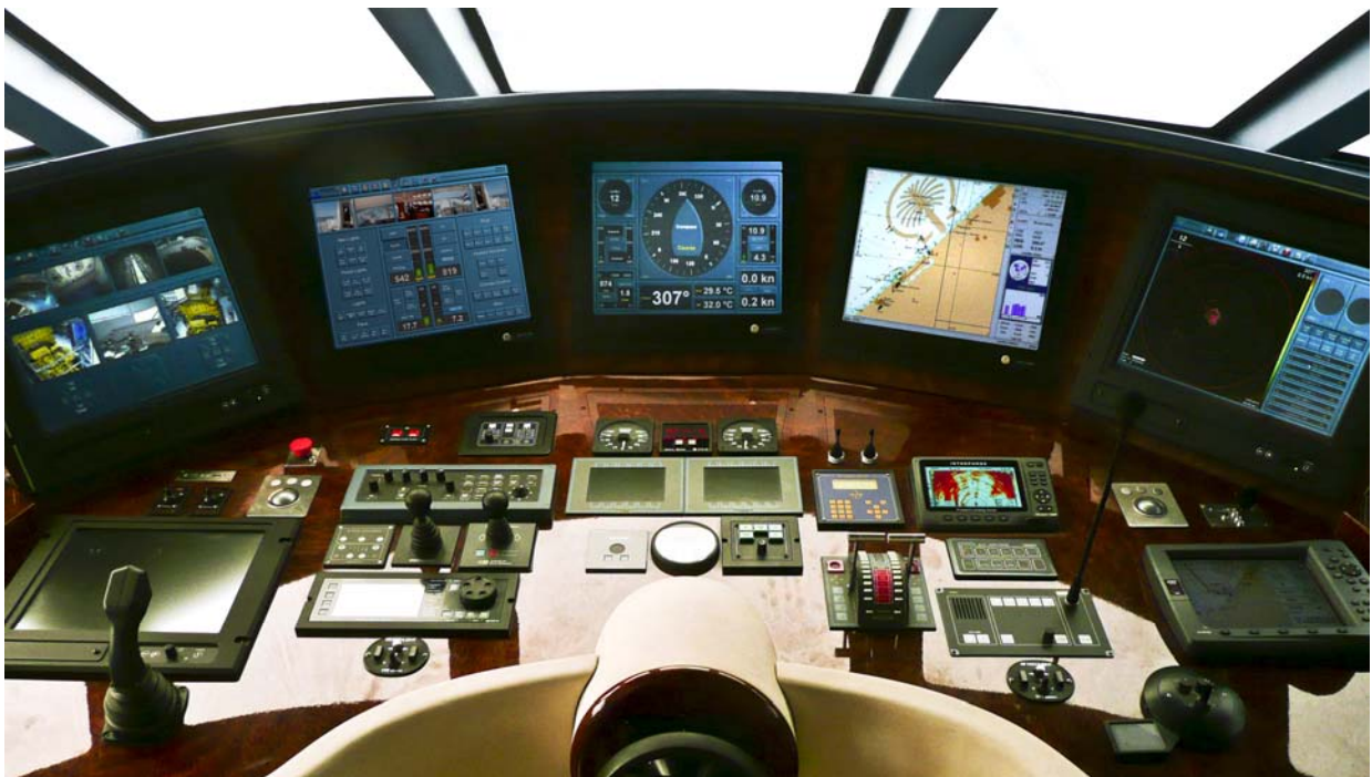
Figure 1-1: Bridge console equipped with FT NavVision® (typical)
