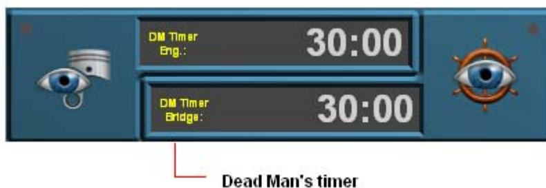
Figure 2-23: Dead Man's (DM) timer
