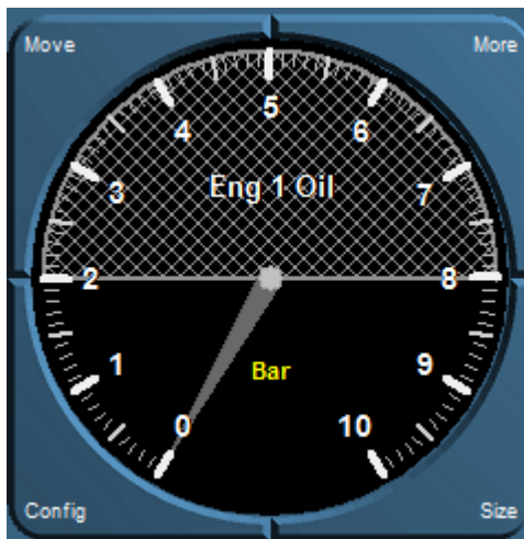
Figure 2-43: Engine 1 oil pressure indicator (0 - 10 bar)
